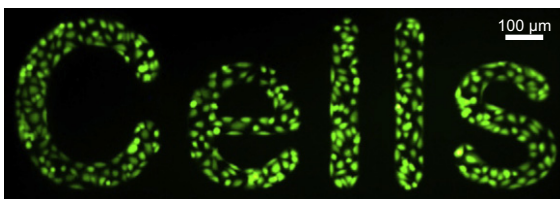
Fig. 6. Confined cell growth in a Petri dish coated with the cell repellent hydrogel agar. The agar layer was selectively dissolved after proton beam writing exhibiting the “Cell” shape as area of exclusive cell adhesion. Fluorescence diacetate stained primary human fibroblast cells after 3 days in culture.
