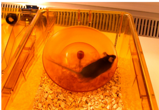
Figure S7. Voluntary Running-Wheel System Photograph of tilted running-track system used for home-cage assessments of voluntary motor-skill learning.
