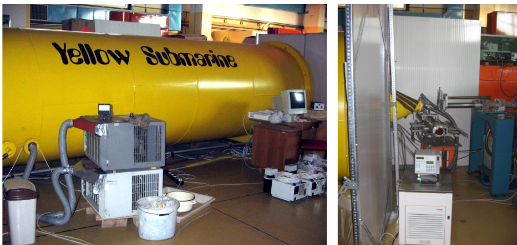
Figure 23: Small angle neutron scattering detector "Yellow Submarine" (left) and automatic sample changer (right) at Budapest Neutron Centre
