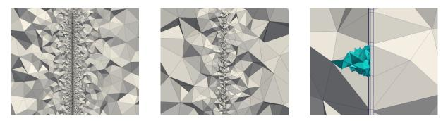
Figure 5.7.: Part of the highly refined primary mesh containing CEM electrodes (left), coarse parameter mesh that reflects a simple discretization for inversion without electrodes (middle) and a selected single region based on clustering (right).
