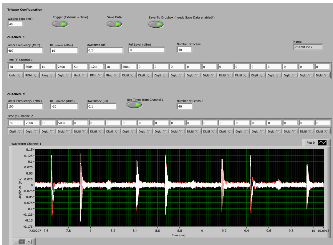
Figure 3.9.: Front panel of the LabView VI used to control the spectrometer. Here we measured spin echoes at 62 Tesla using a \pi/2 pulse of 800 ns and a refocussing pulse of 1.2 \mu s, reflecting a compromise between optimal pulse length and spectral breadth. In this example, the second channel was not used; its settings can be ignored. Immediately after the experiment, the full trace of the signal analyzer is visualized in a simple plot. All post-processing is done with Matlab or Python.
