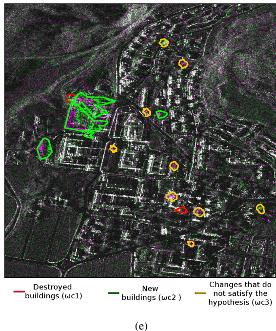
Fig. 13: Trento (Italy) data set: (a) optical image (2011 [36]); and (b) RGB multitemporal composition of spotlight TerraSAR-X and TanDEM-X images (R:03/04/2013, G:21/01/2011, B:03/04/2013). (c) Change detection map M^{\text{opt}} obtained at the level N - 1 = 3 . (d) Map showing the index of the size of changes C . (e) Changed building map overlapped to the RGB multitemporal composition of CSK data.
