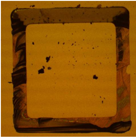
Fig. 1 Fractured sealing ring residues on Au substrate after removing the cap during the shear test.
