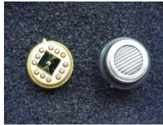
Figure 1. Packaged gas sensors. It is gas sensing nano-material (Pd-doped Tin dioxide with particle size of about 10nm) deposited on MEMS substrate.
