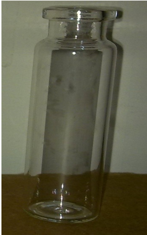
Figure 4.5: Glass vial used for the evaluation of CO 2 produced by yeasts.
