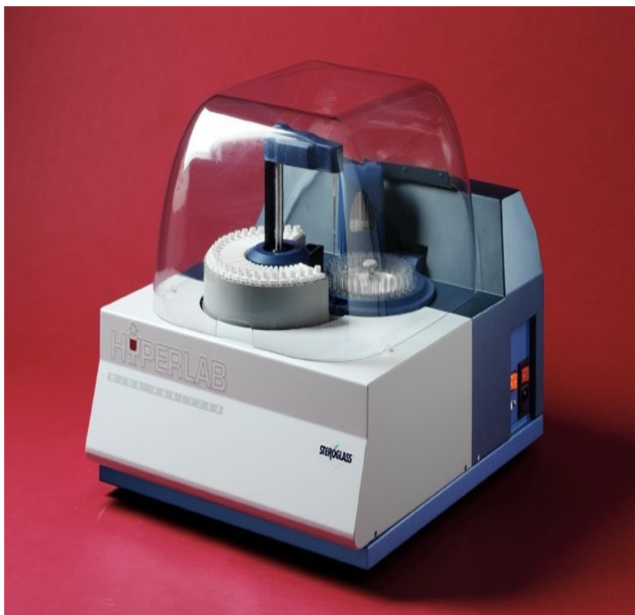
Figure 4.10: Hyperlab automatic multi-parametric analyzer.
