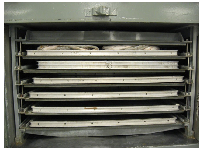
Figure 2. Two fish blocks in a contact thawer, a converted horizontal plate freezer.
