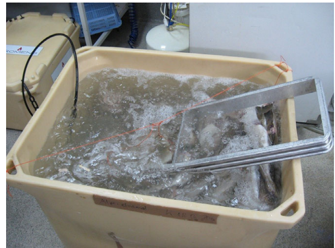
Figure 1. Fish blocks under air-assisted thawing in a 1000 L fish tub. The air bubbles were generating circulation for enhanced overall heat transfer.
