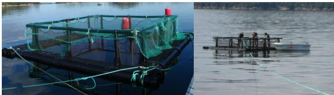
Figure 2. Net pen used in the experiment (left) and during towing (right). Experienced personnel from Austevoll research facility was observing fish during towing aiming to avoid the fish getting stressed.
