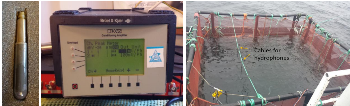
Figure 5. Hydrophone (left) and amplifier (middle) and positioning of hydrophones in net pen (right). The depths for the two hydrophones were 3 and 5 m.
