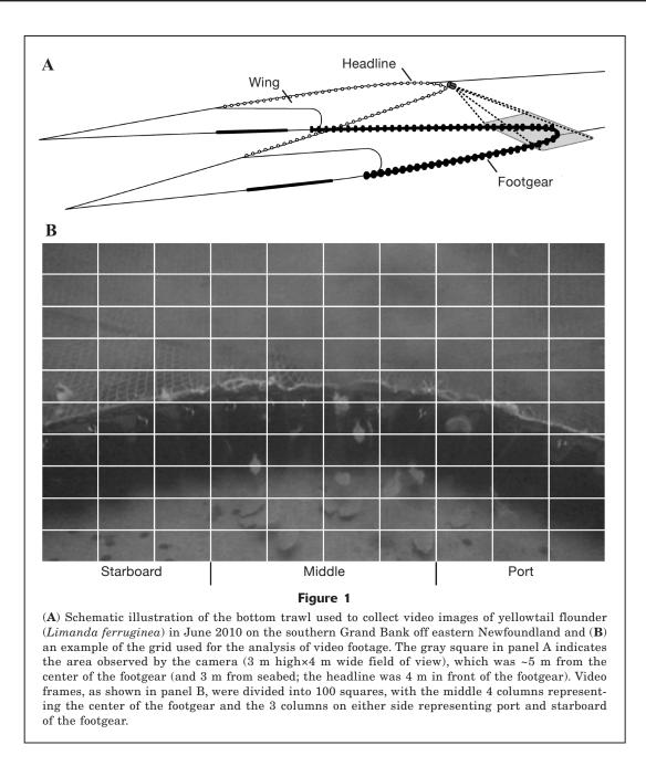
and durations of tows were in a range of 2–3 h. Tow direction was decided by commercial operations and was different for each tow. The height of the headline was approximately 3 m and was recorded with a sensor (Marport Stout Inc., Snohomish, WA) attached to the headline on all tows without the use of camera documentation during the cruise. The door spread ranged from 113 to 123 m and was measured with spread sensors (Marport Stout Inc.) placed on the trawl doors.
