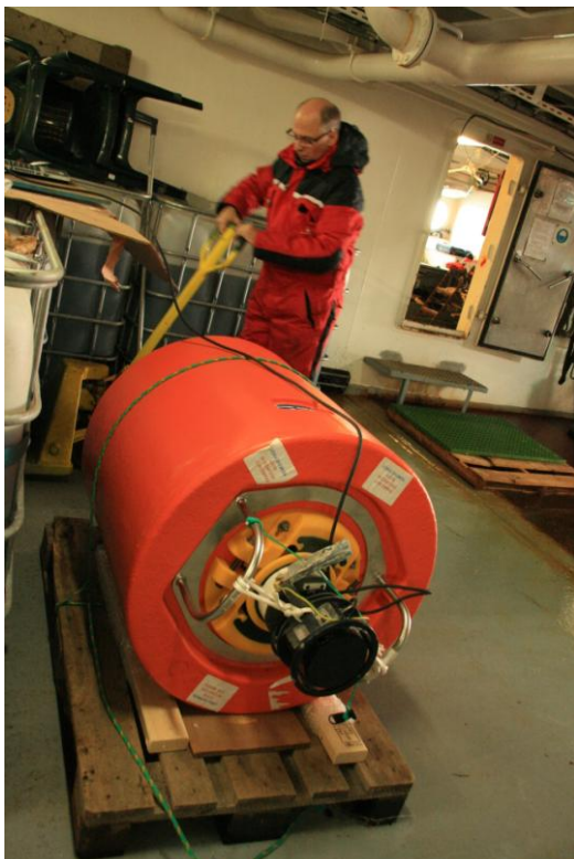
Figure 2. Acoustic mooring mounted inside the company designed original frame. This frame was used when the mooring was redeployed for a new year of logging, but not during the 1-year period it had already been deployed.
