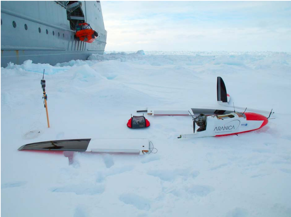
Figure 14. CW1 disassembled and ready to be packed in a container and picked up by the ship. Photo: M. Poltermann
