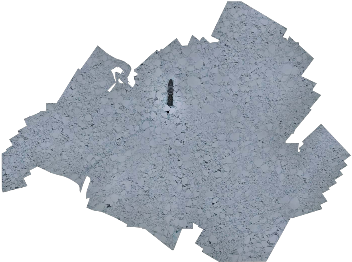
Figure 6. Mosaic from CWM flight on the 19 March. As the flight was mainly flown in manual mode due to airspeed sensor issues no structured grid was flown. The mosaic is based on 300 images from a 15 minutes flight.
