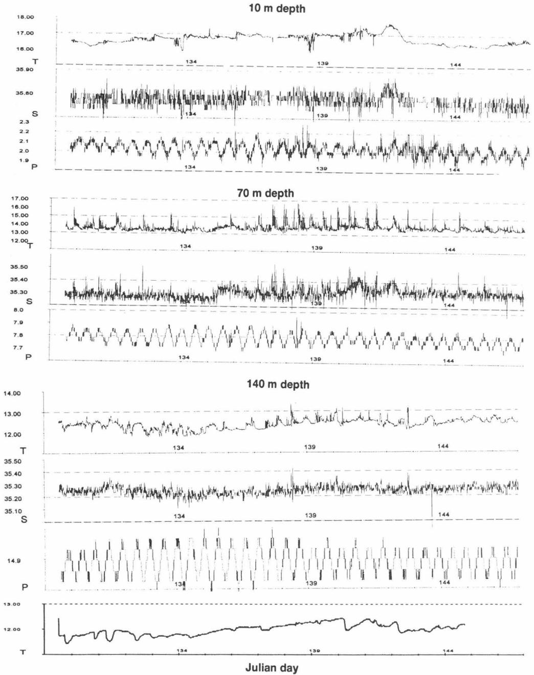
Fig.4 Temperature, salinity and pressure from the 3 current meters versus Julian Day. The lower panel show the temperature observations from the water level recorder at the bottom at 170m depth.
