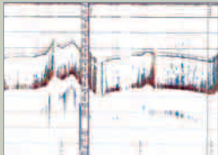
Simultaneous echograms, with and without the protruding keel, in bad weather.
