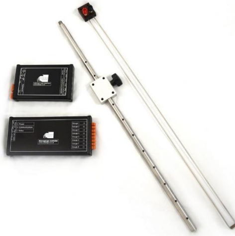
Figur 28 Edinburgh Designs WG8USB Wave Gauge Controller med probe. http://www.edesign.co.uk/product/wavegauges/
