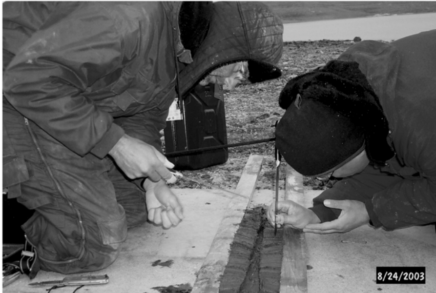
Fig. 6.2-1: Surface sediment core from Duck Lake. The dark horizons are formed by 1-2 cm thick moss layers.
