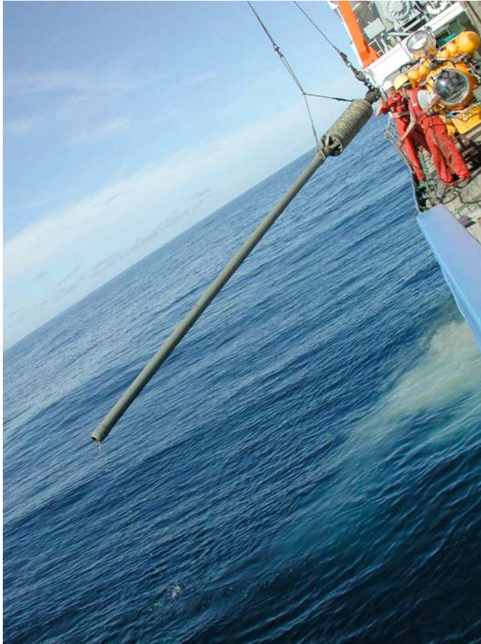
Fig. 5. Gravity-corer with a 6 m barrel.
