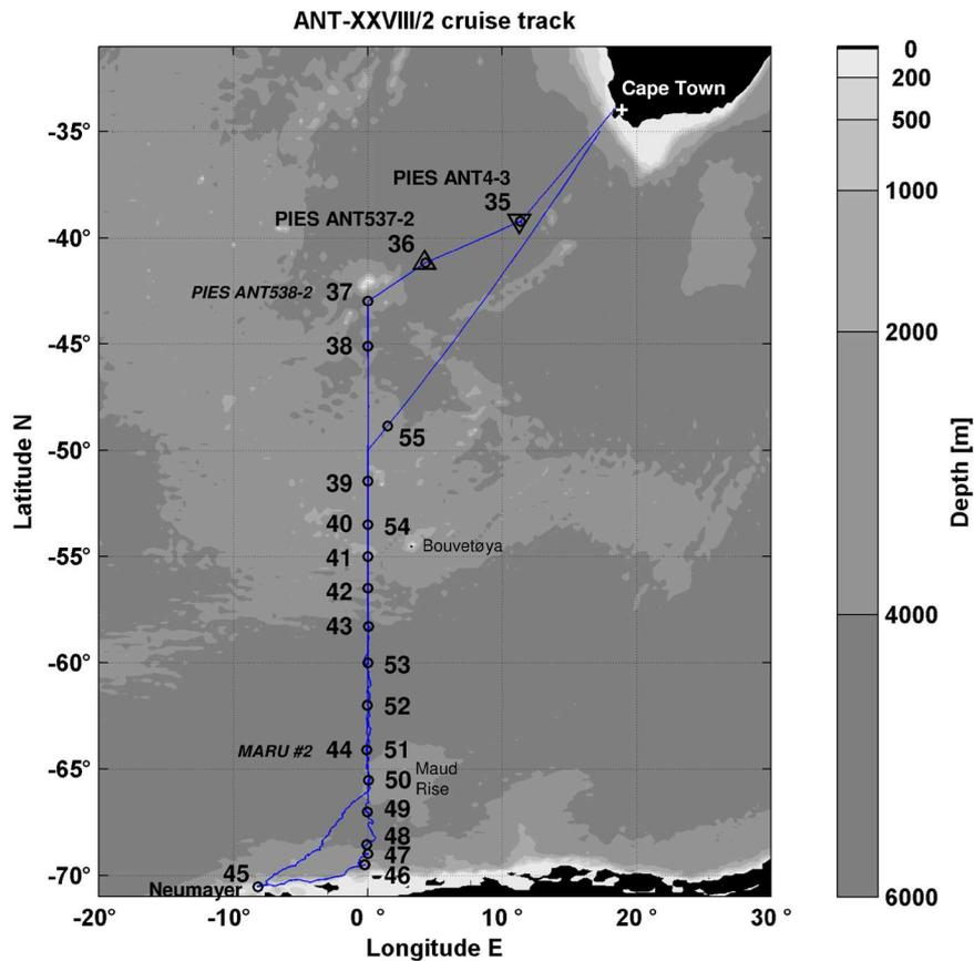
Fig. 3.1: Cruise track of ANT-XXVIII/2 with CTD stations and moorings. Stations are marked by black circles and the corresponding PS79/0xx station number. Mooring deployment is marked with  $\nabla$ , recovery with  $\triangle$ . Unsuccessful mooring recoveries are marked by mooring name only.
