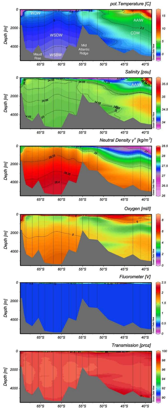
Fig. 3.5: CTD section, full depth range. Black lines denote location of CTD profiles. AAIW Antarctic Intermediate Water, CDW Circumpolar Deep Water, WDW Warm Deep Water, WSDW Weddell Sea Deep Water, WSBW Weddell Sea Bottom Water.
