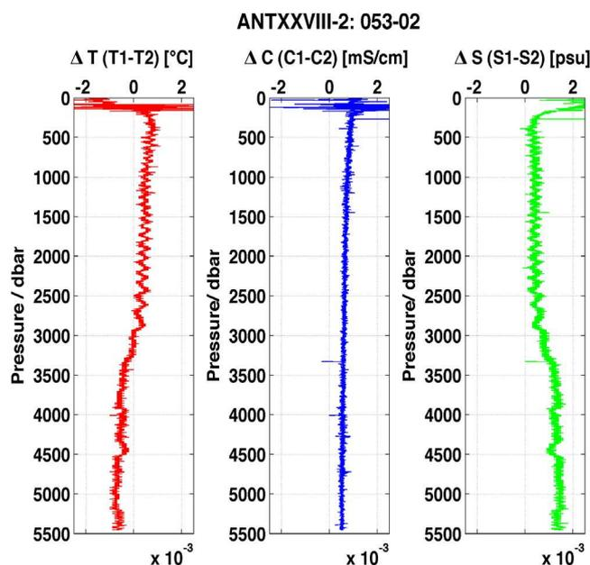
Fig. 3.2: Sensor differences  $\Delta T = T_1 - T_2$ ,  $\Delta C = C_1 - C_2$  and the difference between salinities derived from each sensor pair at station 53-2. Oscillations correlated with rosette rotations show up most pronounced in the 1500 to 2,500 m depth range.
