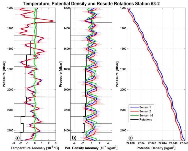
Fig. 3.3: Temperature (a), and Potential Density (b) anomalies. Blue: Sensor 1, red: Sensor 2, green: Difference Sensor 1 – 2. Black: Rosette rotations \*0.2. Heavy lines: Band-passed anomalies showing only variability with length scales between 25 dbar and 250 dbar. Light lines: 1 dbar data. (c) Profiles of absolute Potential Density, with rotation-related wiggles clearly visible.
