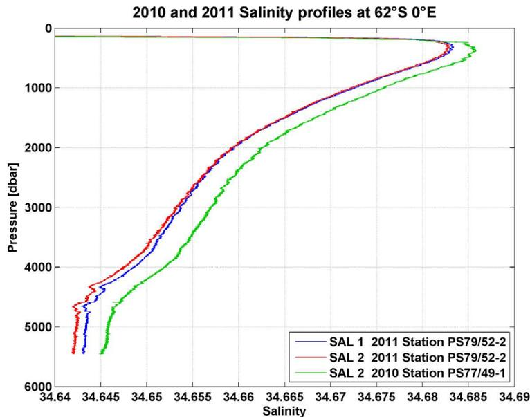
Fig. 3.4: Salinity profiles at 62°S 0°E. 2011 profiles shown in blue (Salinity 1) and red (Salinity 2). The 2010 profile (green) is Salinity 2, which better agreed with the salinometer calibration in 2010. Note the reduced offset of SAL2(2011) to SAL2(2010) in the deep part of the profile. The small wiggles around 1200 m to 2500 m depth can be attributed to the rotation-related temperature oscillations.
