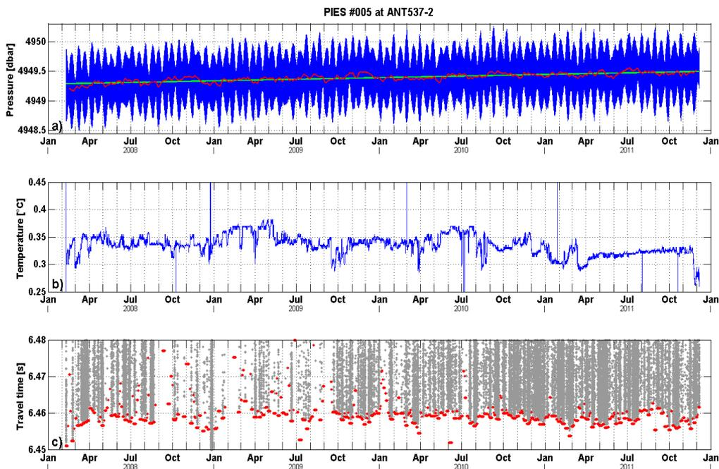
Fig. 3.10: PIES ANT538-2 time series. Figure shows uncorrected raw data. a) Pressure, hourly data (blue), 7 day low passed values (red), linear trend (green line). b) Near-bottom temperature. c) Acoustic travel time (grey dots). The travel times shown represent 6 % of all pings only; in 94 % of all pings no echo was detected. Minimum travel times in 7 days intervals shown in red.
