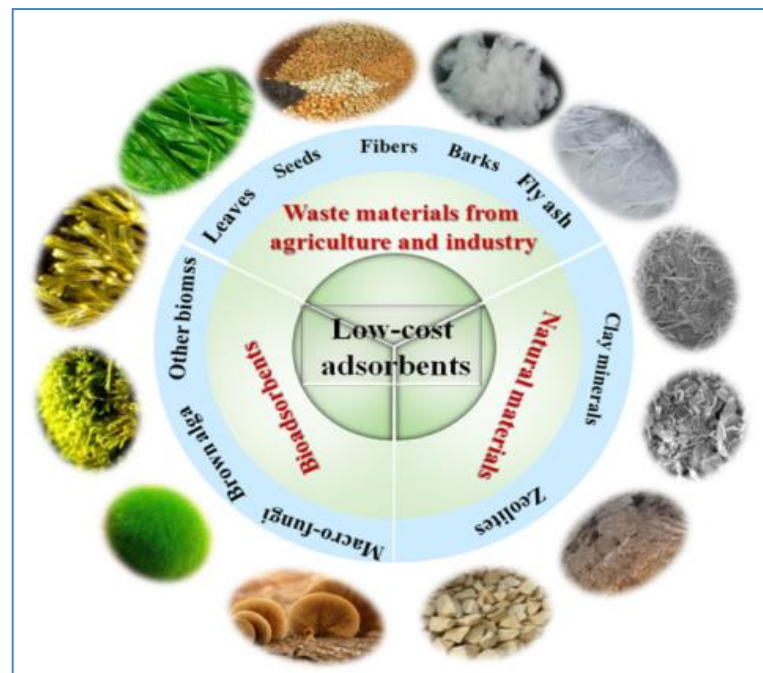
Figure 2-3: Common low-cost adsorbents for pollutants removal from water (Mu and Wang, 2016)
