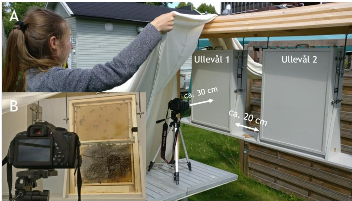
Figure 2 The bee hives Ullevål 1 + 2 and the camera are about to be covered with an awning (A). Once the awning is on top of the hives, the lid of the hives could be opened and the filming process of the dances on the lower frame could start (B).
