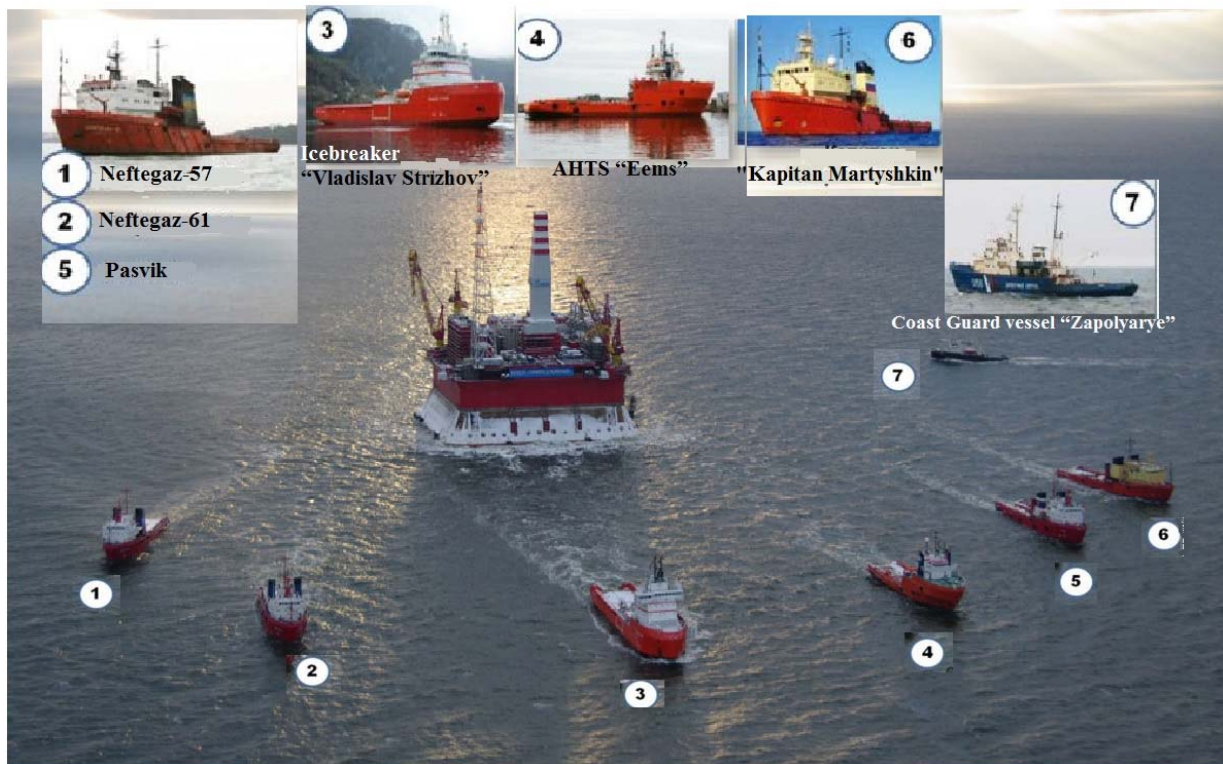
Figure 43. The towing operation of the Prirazlomnaya platform in August 2011 (Source: by the 1 st author based on Gazpromneft data)
