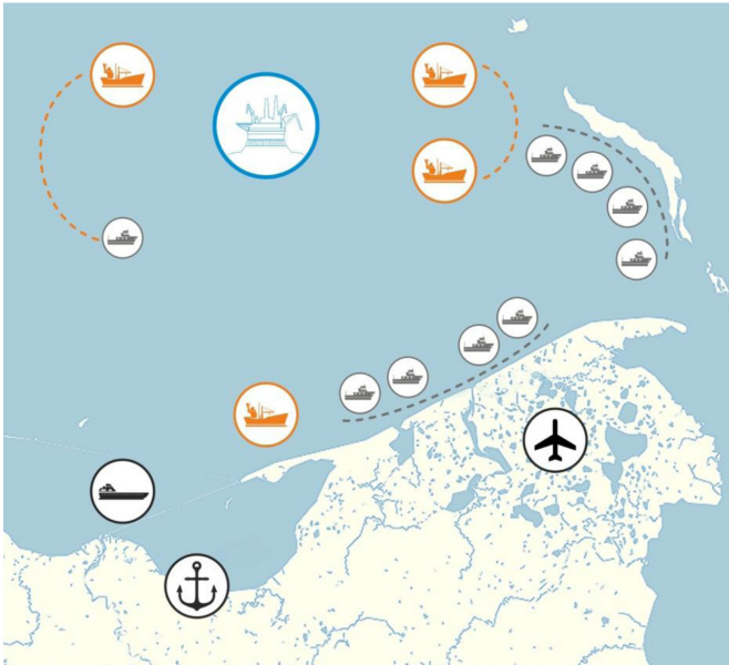
Figure 3.1.2. Alignment of response resources, “Prirazlomnaya”. Source: Alexander Mandel, GaspromNeftShelf (ice-breakers in orange, boom boats in grey, tanker in black).
