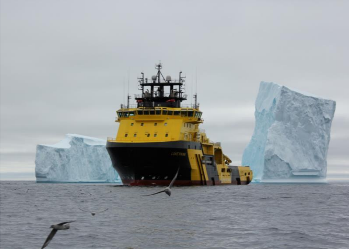
Figure 18. Balder and Vidar Viking are sister ships and examples of icebreaker AHTV.
