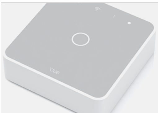
Figure 17 – Gateway for communication between AMS, relay and computer[40]
