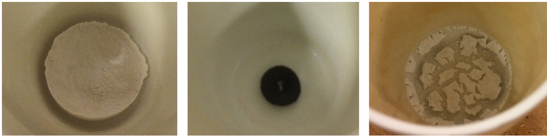
Figure 4.1.1: Remaining ash in crucibles after test 1. S. platensis (left), C. vulgaris (center), P. tricornutum (right).
