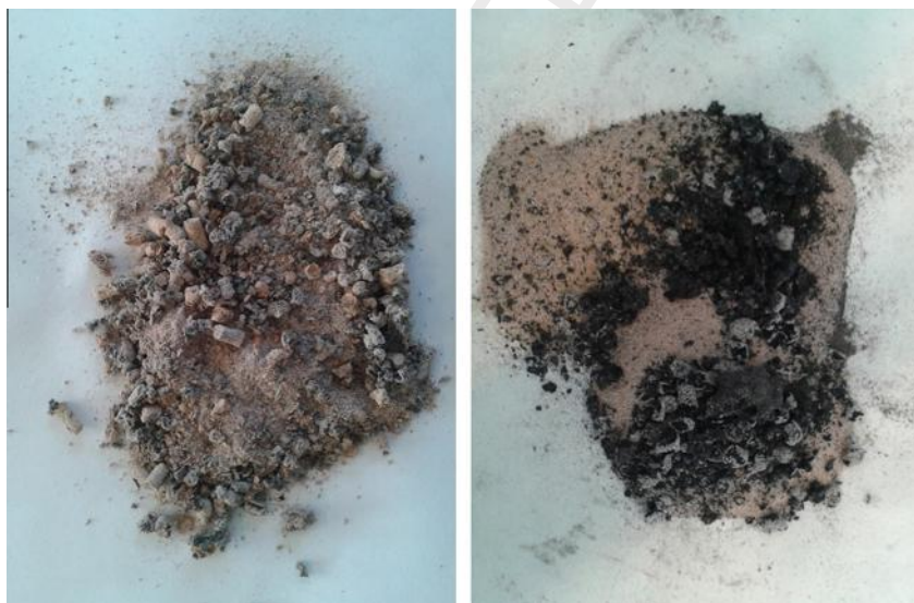
Fig. 2. Residual char, ash and bed-material from the gasification tests (left: alfalfa, right: wheat straw).
