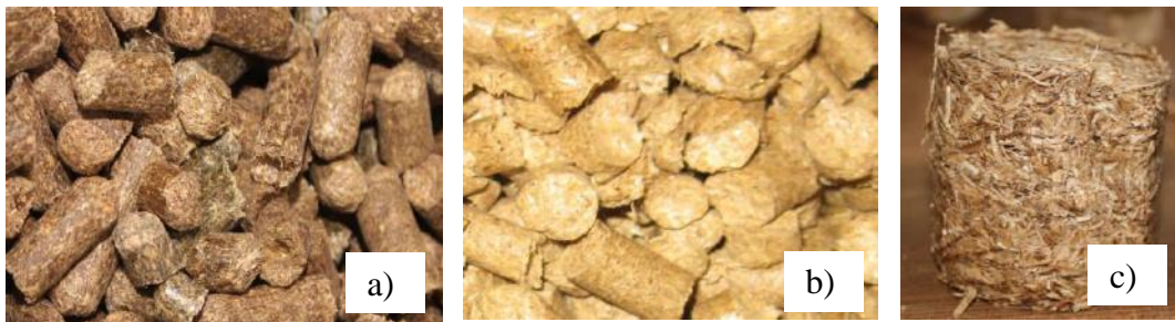
Figure 3.3: Biomass pellets and briquettes for gasification tests (a): alfalfa pellets, b): wheat straw pellets, c): common reed briquettes
