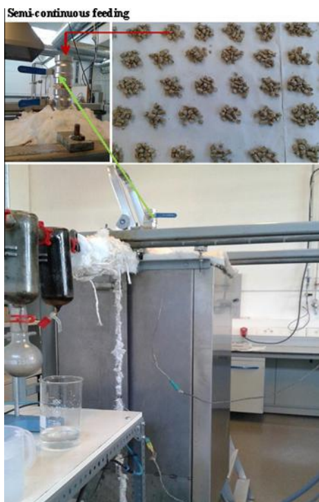
Fig. 3. Semi-continuous feeding with two valve assembly.
