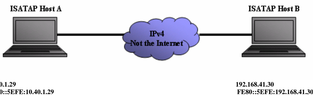
Figure 4.11: ISATAP on IPv4 (not the Internet).
