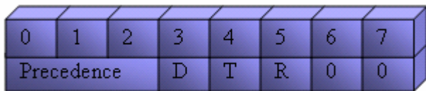
Figure 2.2: The Type Of Service field.
