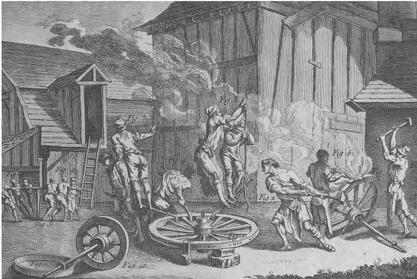
Figure 2.13: Plate depicting two methods of shoeing a wheel. In the centre the labourers are using hammers and "devils" to fit a hoop onto the rim, and on the right they're hammering strakes into place. Published in a volume of Encyclopédie in 1769 Diderot and Rond d'Alembert 1769.
