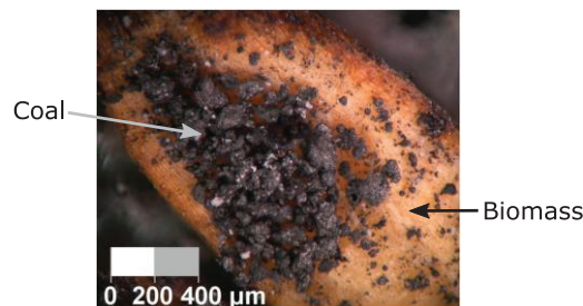
Figure 3. Example of particles gathered from a co-firing flame. The black coal particles are clearly much smaller than the white biomass particles on which they are positioned.
