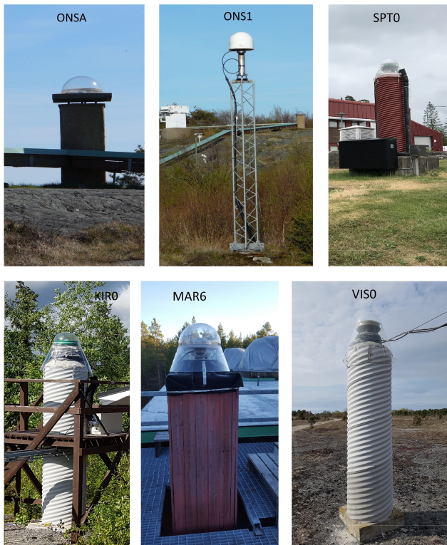
Figure 2. The six antenna installations used to acquire the GPS data. See Fig. 1 for their geographical location.
