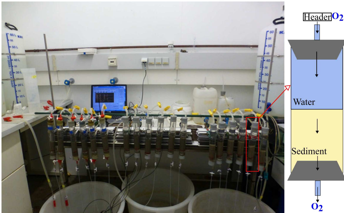
Figure 7: Flow-through cores in the lab, the principle of each core was depicted in the zoomed drawing. Oxygen concentration was measured in the header and in the outflow of each core (indicated by O_2 ).
