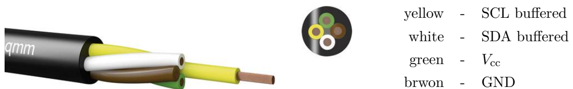
Figure A.5.: LifYDY cable wire assignment.
