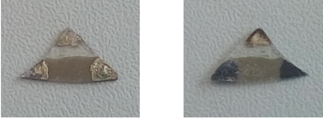
Figure 5.2.3: Photography of a titanium dioxide thin film sample after the resistivity measurement in vacuum from the front (left) and the rear (right). The electrical field was applied tangential to the surface between two electrodes. The third electrode is a blind electrode which was not connected.
