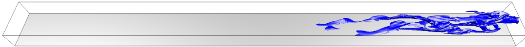
Figure 5.6: Example of large-scale vortex structure in open duct flow with A = 1 and Re_b = 2205 ; flow direction is from left to right. The vortex was educed by \omega_x^{\pm} = -0.16 .
