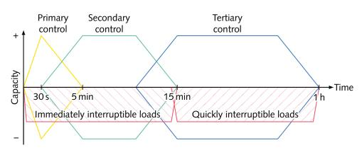
Figure 2.6 | Chronological sequence of the usage of the operating reserves and interruptible loads. Transmission system operators have three different reserves at their disposal, which can be utilized successively if a power imbalance occurs. Additionally, since the amendment to the Energy Industry Act of 20 December 2012, quickly or immediately interruptible loads can be accessed if negative balancing power is required.
