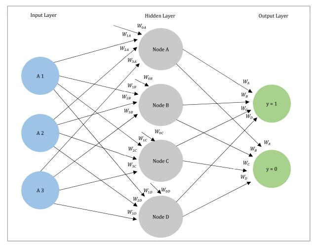
Figure 14. Neural Network model with one hidden layer, based on Larose et al. (2015: 341).
