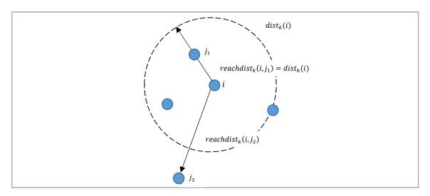
Figure 9. Concept of *reachability distance* for *k* = 4 based on Breunig et al. (2000).
