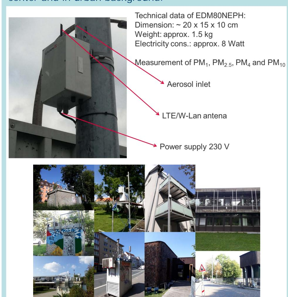
Calibration of the Scientific Scouts by comparison with a reference measurement device (Grimm EDM164):
