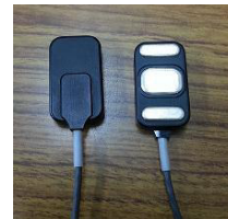
Fig.4: Sensor used for EMG measurement [14].
