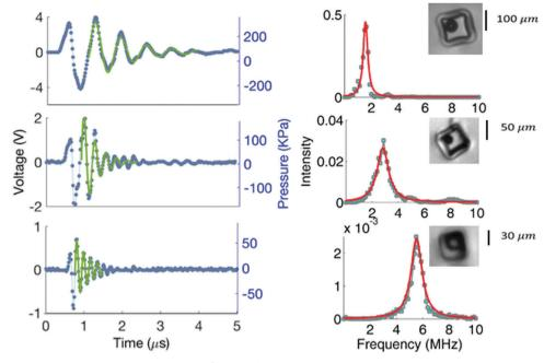
**Fig. 4** Acoustic signals captured with the proposed method. On the left column: Pressure waves emitted by a bubble nucleated in three cubic cavities with size  $L_c = 100-50-30 \mu m$  from top to bottom, respectively (blue dots); curves (in solid green line) obtained by substituting in eqn (16),  $\omega_0$  and  $\tau$ , found by fitting the frequency-domain signals (17). On the right column: Power spectra density (light blue filled squares), fitted with eqn (17) (solid red line).
