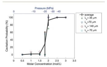
**Fig. 2** Cavitation probability curves as a function of the salt molarity (bottom *x*-axis) and liquid pressure  $p_1$  (top *x*-axis) for four samples with different cavity size. The averaged curve is represented in grey.
