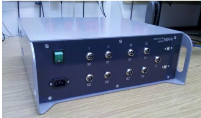
Fig. 8. A photo of a two-bit quadruple three-phase power analyzer (MM4).
