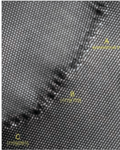
Figure 1 The boundary in \{110\} mazed bicrystal with 3 major facet inclinations.
