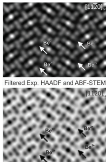
Figure 3. Filtered HAADF-STEM and ABF-STEM images of taaffeite \text{BeMg}_3\text{Al}_8\text{O}_{16} .
