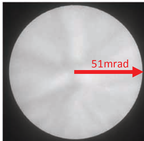
Figure 2. 40kV Ronchigram with 51mrad convergence semi-angle.
