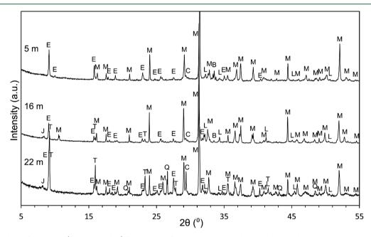
**Figure 2.** Typical slag diffractograms (from borehole 1) from depths of 5, 16, and 22.5 m, with assigned mineral phases. Key: M, melilite group minerals (gehlenite and åkermanite); E, ettringite; Q, quartz; C, calcite; L, larnite; B, brownmillerite; T, thaumasite; J, jenite.
