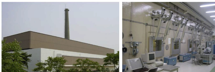
Fig. 1. Chemical Processing Facility (CPF) of JAEA. (Left) Appearance of the facility, (Right) Hot cells for reprocessing experiments.
