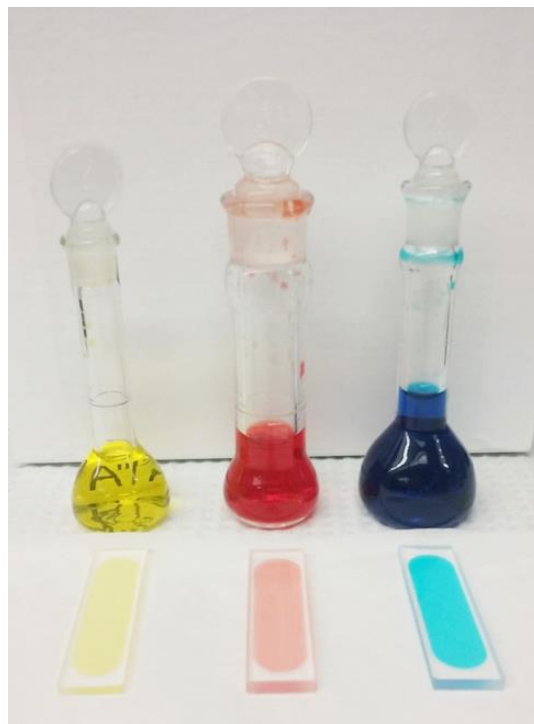
Fig. G1. Individual color additive molecules mixed in ethanol solvent with corresponding 0.1 mm path length cuvette sample preparation. From left to right: FD&C Yellow No. 5, “Tartrazine”; FD&C Red No. 40 “Allura Red”, and FD&C Blue No. 1 “Acid Blue 9”
