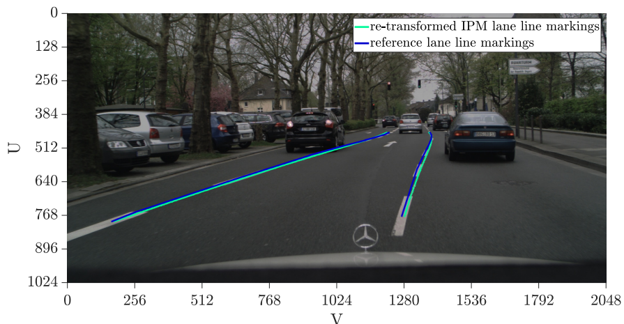
Fig. 2.11 IPM lane line markings re-transformed into the camera image and compared to the reference lane line markings for the ego-vehicle lane.
