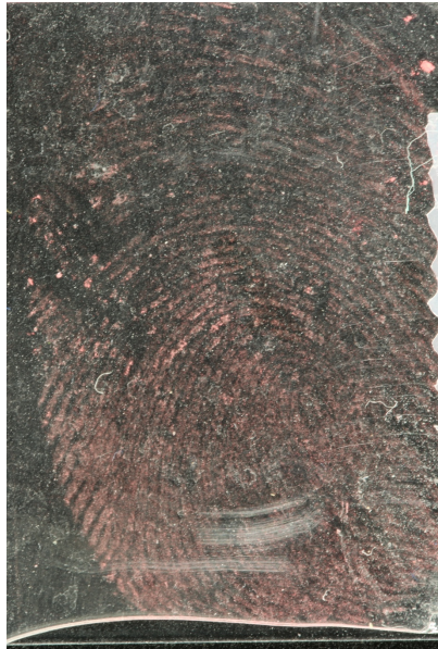
Figure 3: Photograph of a developed dirty fingermark lifted from glass. These marks showed great ridge detail and detection of cocaine using these marks was possible.
