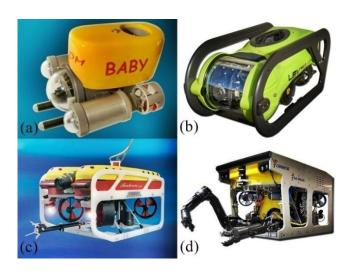
**Figure 2.2:** Example of different types ROV (a) micro ROV (GNOM, 2012), (b) mini ROV (Seabotix, 2012), (c) general ROV (SAAB Seaeye, 2012) and (d) work class ROV (Nautic Expo, 2012)
