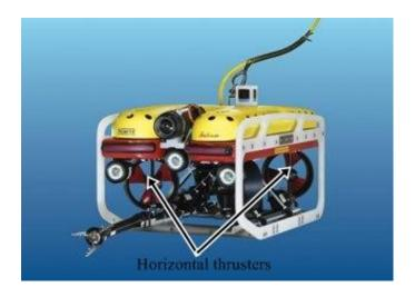
**Figure 1.3:** Example of horizontal thrusters configuration on Seaeye Falcon ROV (SAAB Seaeye, 2012)
