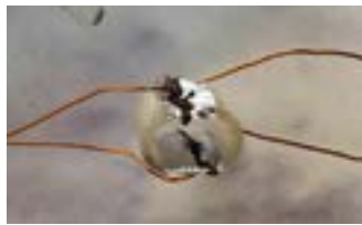
Image 6. A typical crush wire contact. Several dozen switches like this may be present on lengths of lacquered wire up to 10 m in length. 7
